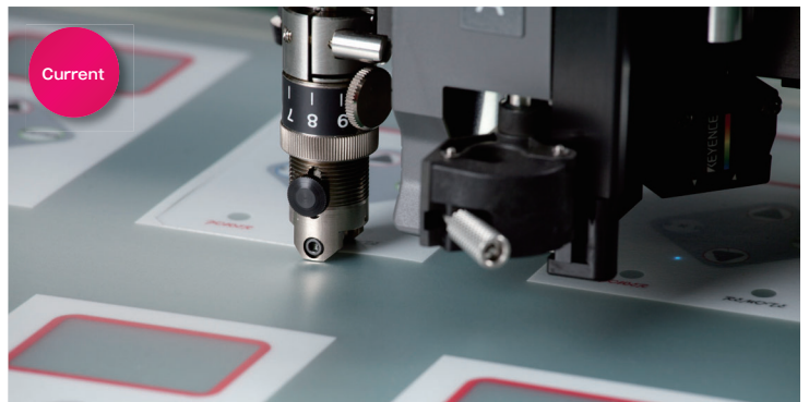
Cutting the sheet to size is made possible via our cutting plotter machine, thus cutting die manufacture process can be eliminated.
