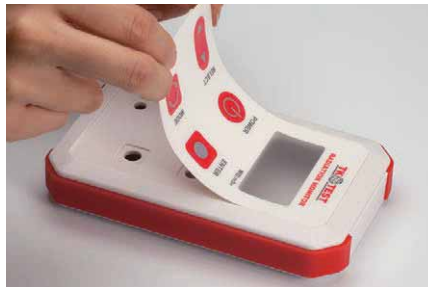
8. Sticking overlay sheet onto enclosure
