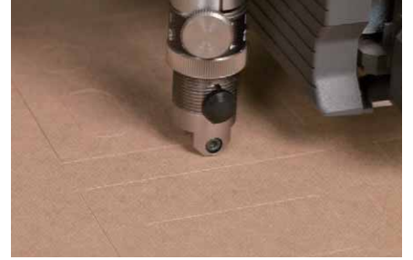
3. Cutting double-sided tape
