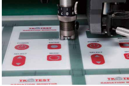
5. Cutting the sheet to size
