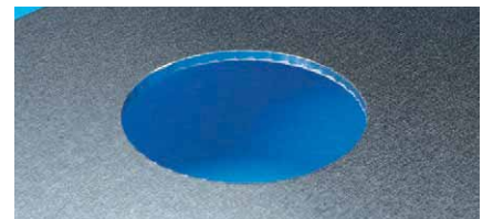
Punching of large circular holes with multiple smaller die strokes.
