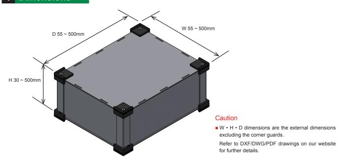
■ Panel thickness, screw sizes, and pillar types vary by W / D dimensions.
