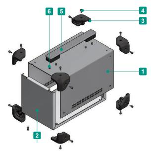
Aluminium case and corner guard with screw fastening.
