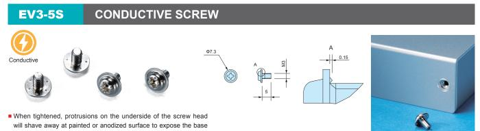
When tightened, protrusions on the underside of the screw head will shave away at painted or anodized surface to expose the base material for achieving conductivity.
