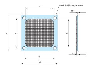
■ Use for EMC shielding on the hole for cooling fan.
